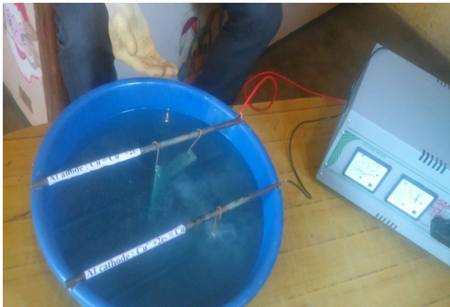
Fig. 4: Setup of electroplating
